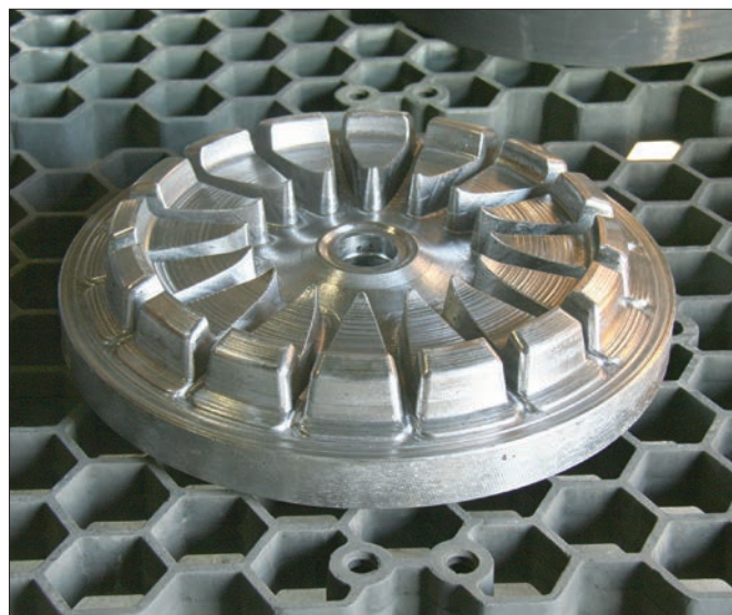
A lower die for aluminium rim just before heat treatment on charging grid. Photo: ASSAB Çelik (Turkey)
