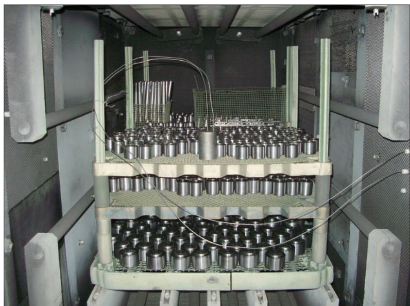
The use of thermocouples gives an overview of the temperature in different areas during heat treatment. Photo: Böhler Uddeholm Czech Republic
