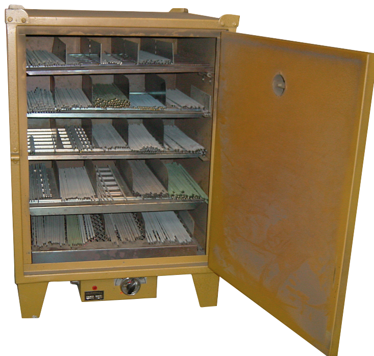
Dry cabinet for storage of electrodes.
