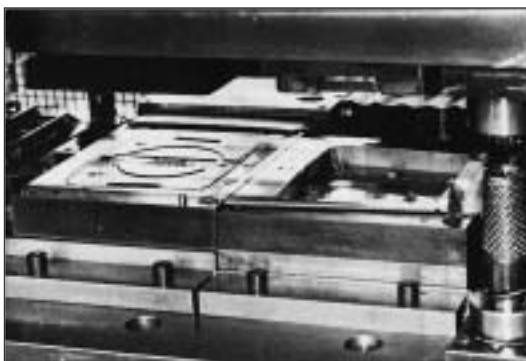
This tool was made from Rigor. 3 million parts were manufactured before the tool was reground.
