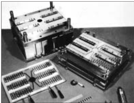
Transfer mould with Rigor inserts to produce encapsulated electronic components.
