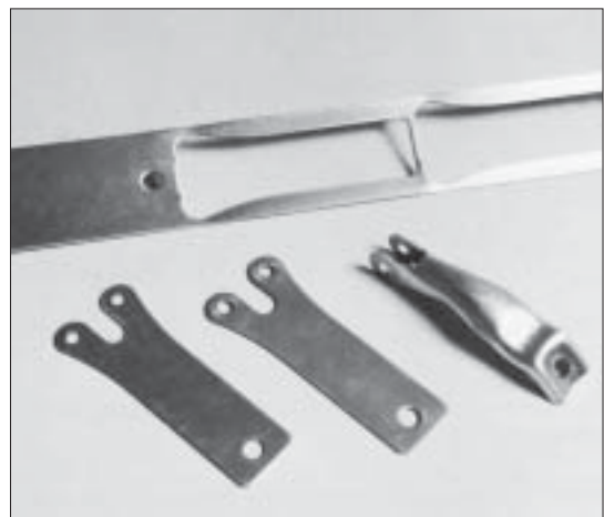
Stainless steel fastener stamped with a Uddeholm Vanadis 23 die and Uddeholm Vanadis 4 punch.
