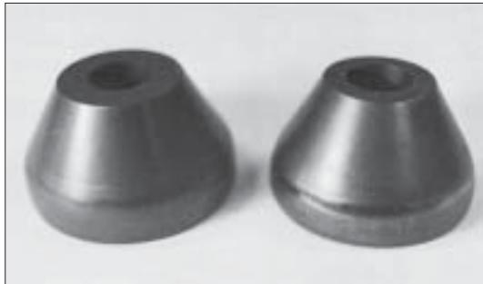
PVD coated tools in Uddeholm Vanadis 23 for cold forming of tubes.
